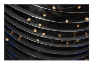
With the rotary spiral separators round seeds can be sorted out from non-round (flat, square, broken, split) material/seeds by means of their rolling features and gravity. The easy to use machines can be delivered with 1, 2 or 4 spiral cores, which are equipped with spiral flights of various sizes and angles appropriate for the required special sorting task. Up to 14 different spiral cores are available used for cleaing fine seeds, spices, all kind of grain, beans and peas, etc.
